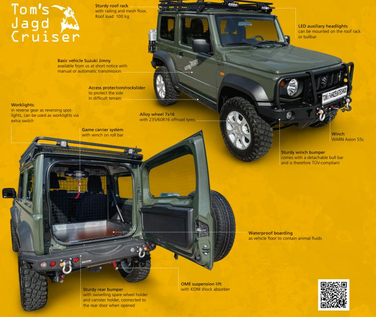
Tom's JagdCruiser: Based on the Suzuki Jimny 1.5. Extremely light, off-road capable 4x4 with ladder frame and rigid axles - unique in this class. Modified by us to become a hunting pro. Put together your hunting vehicle according to your wishes! More details: www.toms-fahrzeugtechnik.com
